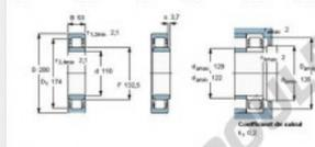
The technical drawing shows a cross-section of the roller bearing. Key dimensions are labeled: d = 110 mm (inner diameter), D = 200 mm (outer diameter), B = 53 mm (width), and r = 37 mm (fillet radius). It also shows the internal structure with rollers and cages, and a note for 'Conditionnement de roulement'.
