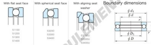
Thrust Ball Bearings - Single Direction
