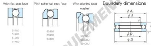
Thick Ball Bearings - Single Direction
